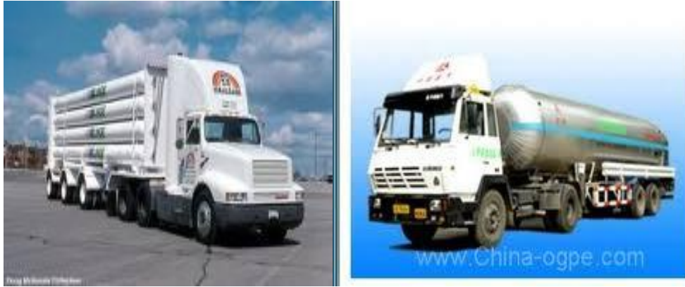
Figure 8: Tube trailer and cryogenic tanker
